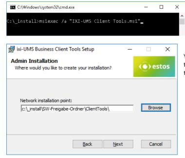
You now have the option to state a directory where the prepared installation shall be deposited. This has to be a shared folder in the network.
