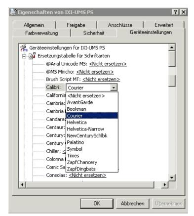
If it is not possible in your environment to change the fonts permanently, a "font replacement" can be entered at the printer.
