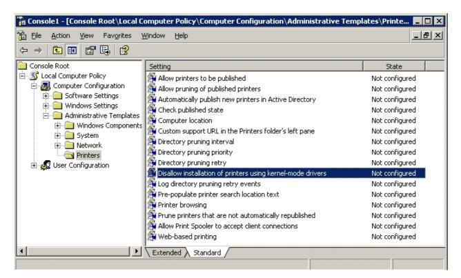
Deactivate the policy "Disallow installation of printers using kernel-mode drivers".
